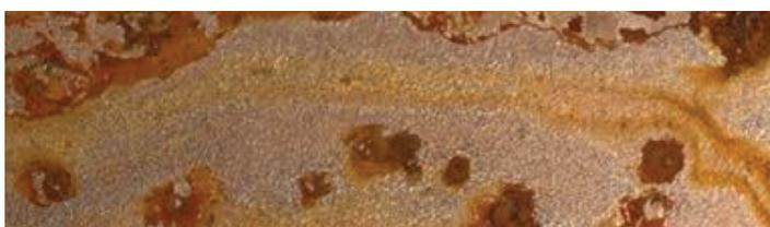
Stainless steel and aluminium alloys are also susceptible to pitting corrosion. These metals have a passive chromium oxide layer on the surface, which keeps them from corroding in a normal environment. If this passive layer is damaged locally, either mechanically or by solutions containing chloride ions, pitting corrosion may occur.
