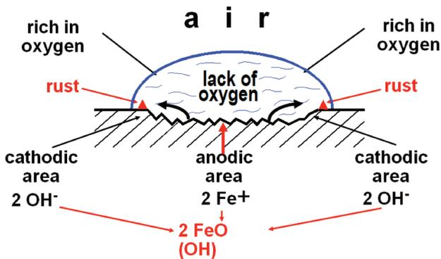
The figure above represents a water drop resting on a plain iron surface. The surface of the water droplet is exposed to air, making it rich in oxygen. The inside of the drop has a lack of oxygen, which creates a difference in electrochemical potential allowing electric current to flow. Electrical current flows through the water, which acts as an electrolyte, from the anodic surface of the iron to the cathodic surface of the water causing iron ions to dissolve.
