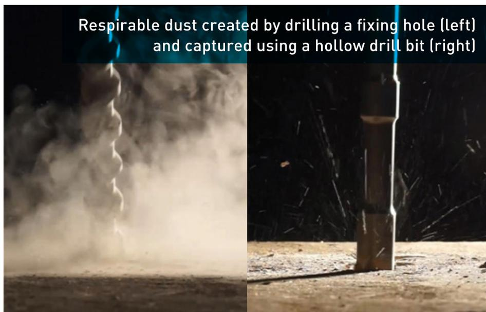
Respirable dust created by drilling a fixing hole (left) and captured using a hollow drill bit (right)
