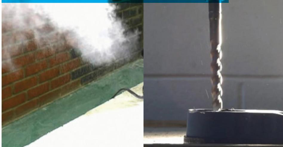
As of this article, the vac connected to the tool must be rated to a minimum of 'M' (medium) hazard class. An 'L' (low) or unrated vac will not be able to capture the very small dust particles and is effectively useless. An 'H' (high)
